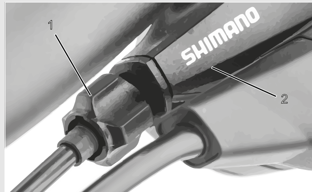
Figure 68: Adjusting sleeve (1) for the single-cable, cable-operated gear shift with shifter housing (2), example
