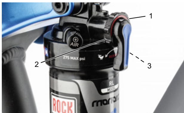
Figure 61: Setting the rebound damper strength on the rear frame damper setting wheel (1)
